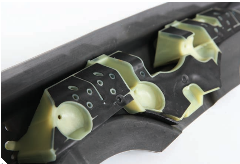
Reinforcer application examples 1 B-pillar junction with roof frame 2 C-pillar application
