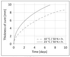
Diagram 1: Curing speed Sikaflex®-295 UV
