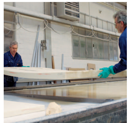
Positioning of the core foam
