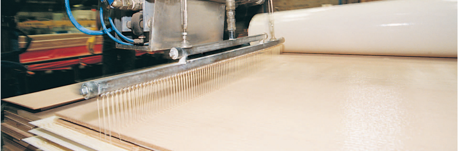
SikaForce® applied by spreader bar
