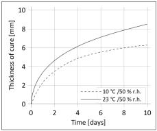
Diagram 1: Curing speed Sikaflex®-552 AT
